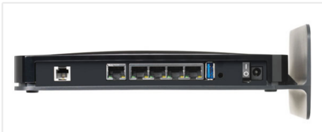
DSL line in, gigabit WAN port, 4x gigabit Ethernet ports, USB port, power switch and power jack. There's another USB port on the front — both are only USB 2.0, despite the blue colouring.
